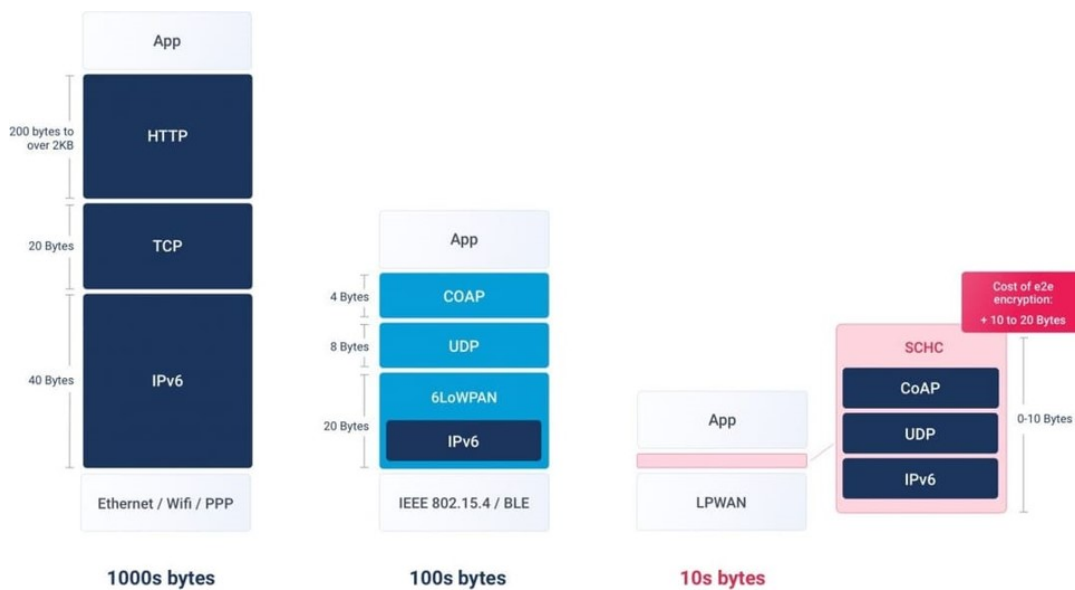
FIGURE 4.1: SCHC compression capabilities (Source [322])
